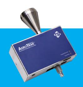
These particle counters can also store up to 3,000 sample records providing data redundancy. Each instrument reports up to four particle sizes simultaneously and other key information such as sensor status, date of last calibration, serial number and date of manufacture for easy warranty management.
